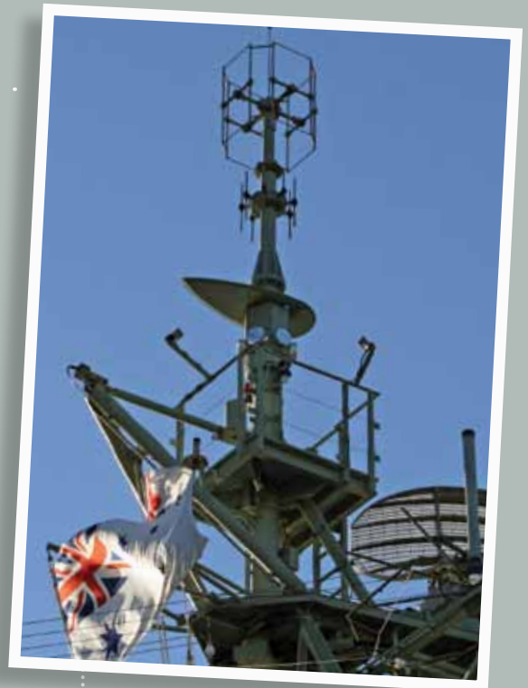
The DSTO-designed radio emission shield (surfboard shape, centre of picture) fitted to HMAS Stuart.
