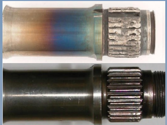
Sea King input drive shafts, showing aftermath of spline shearing at top.
