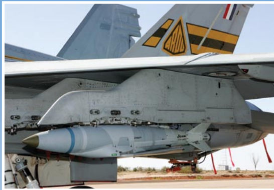
Left: Fluid Dynamic modelling of airflow around F/A-18 fuselage with attached store. Centre: JDAM-ER store carried by F/A-18 during recent Woomera trials of the JDAM-ER device. Right: Scale model F/A-18 with mounted stores for study in DSTO's transonic wind tunnel.
