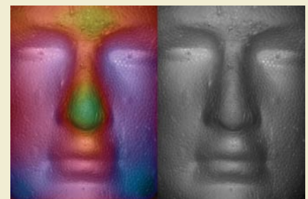
Quantitative phase images of face, with image on left colour-enhanced to highlight depth difference in features.
