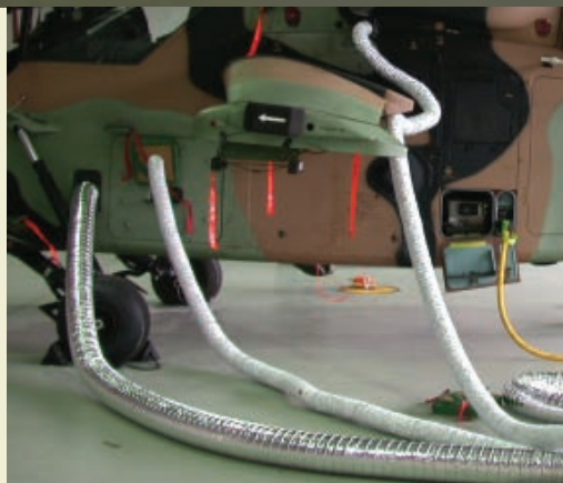
Top and inset: Tiger ARH helicopter in hangar with dehumidification apparatus.
