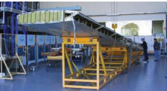
Orion wing under structural test.
