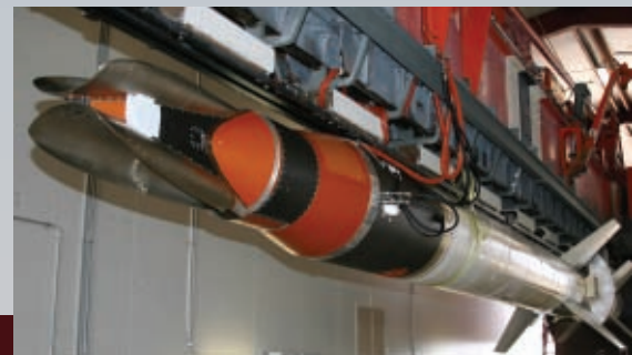
Above left and right: the HyCAUSE scramjet test apparatus and launch vehicle rocket before launch.
