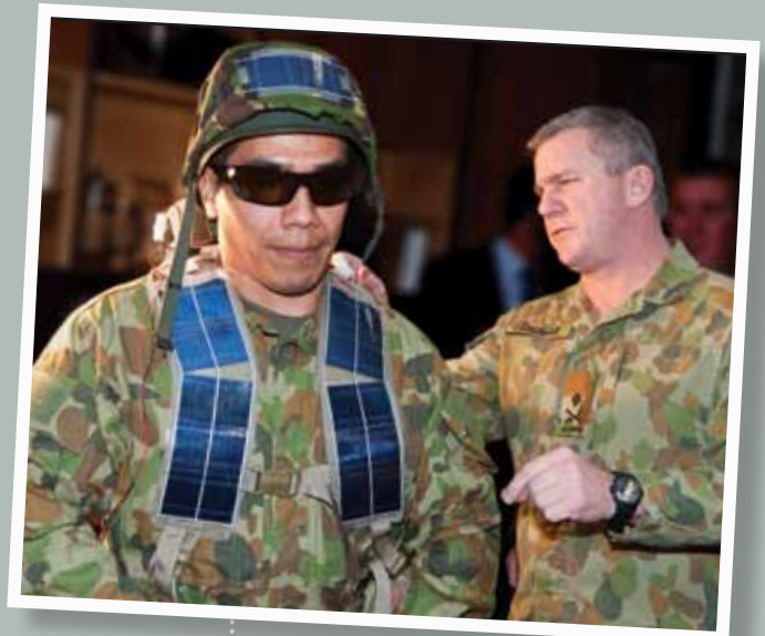
Demonstration version of wearable solar panel technology being developed for Defence by the Australian National University.
