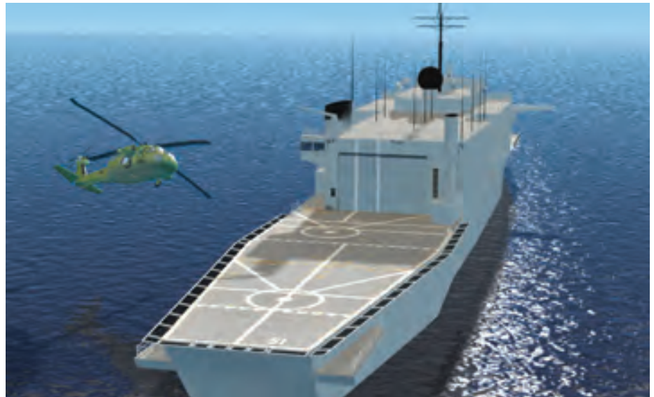
DSTO modelling of Black Hawk approach to HMAS Kanimbla immediately before collision.
