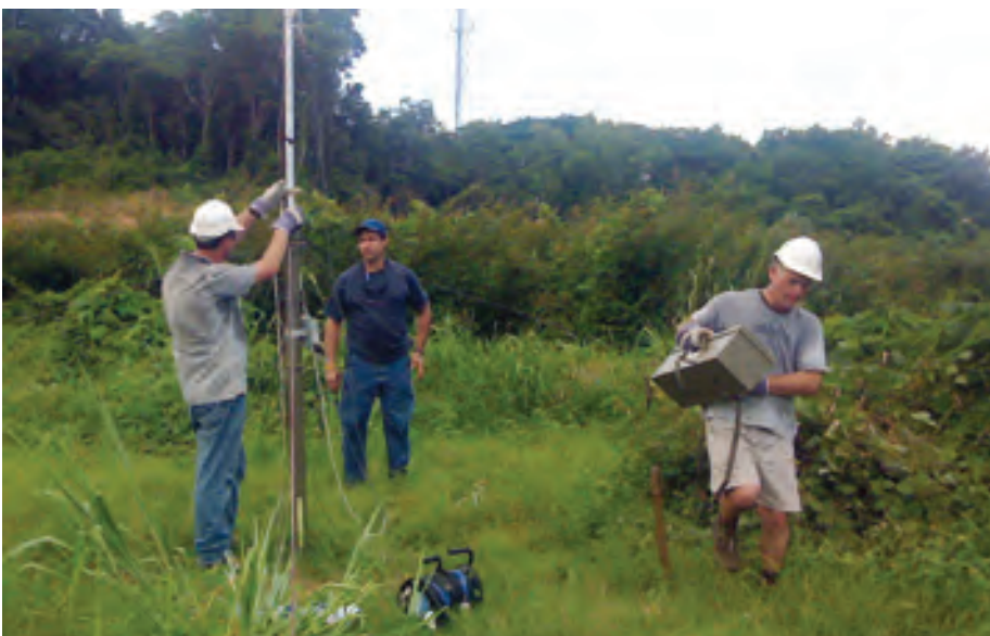
Top of page (inset): Series of ionograms depicting the changing state of the ionosphere measured at a particular time and locality. Background image: US Navy Relocatable OTHR system in Puerto Rico. Above: SpICE research team members erecting an antenna in Puerto Rico for SpICE-3 experiments.
