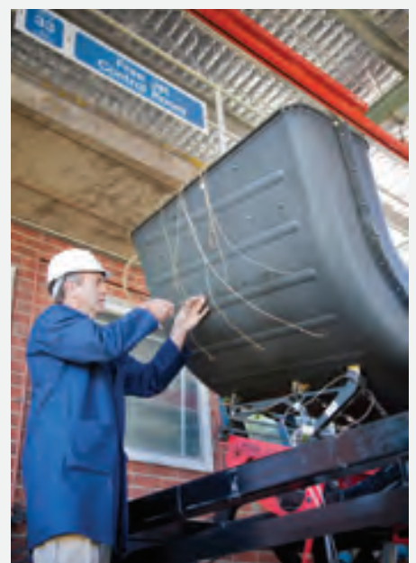
Opposite page and above: Full-scale prototype of Chinook anti-missile countermeasure undergoing testing at DSTO Melbourne.
