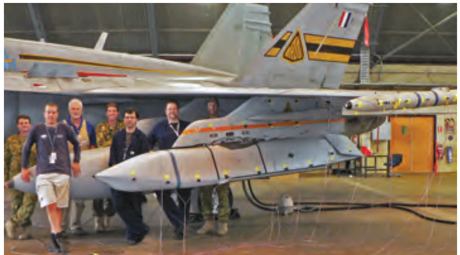
Top: Wind tunnel testing on F/A-18 carrying JASSM. Above: JASSM mounted on F/A-18 for ground vibration testing.
