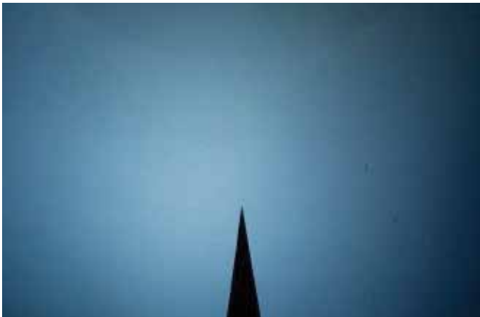
Experimental simulation of pilot's view of helicopter main rotor disk. The rotor tip undersides are painted fluorescent orange-red, but the rotor disk is visible only indistinctly at top of screen when lit just from overhead with natural daylight. The pointer at bottom of image is to be placed by test subjects at estimated edge of rotor tips.
