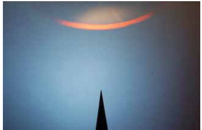
The same scene but with rotor tip undersides illuminated by spotlight. This level of contrast, devised as a control condition for experimental purposes, was not attainable under real-world daylight conditions. Despite the artificially high-level contrast, test subjects performed even worse at judging distance to rotor tips than under lower contrast conditions.
