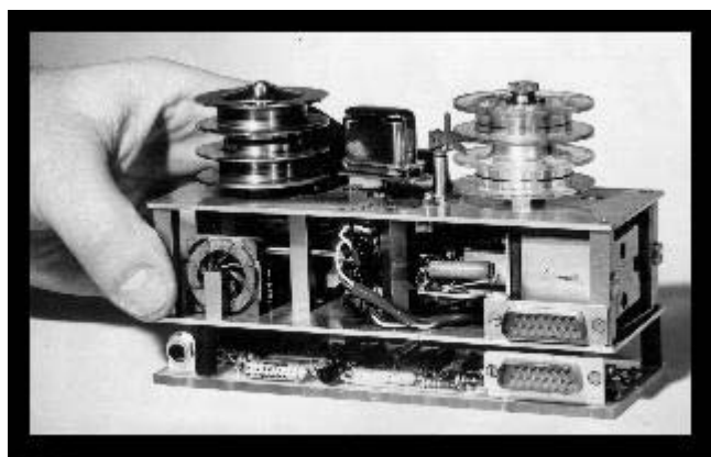
Figure 1: The original (1958) ARL Flight Memory Recorder, capable of storing the cockpit speech and eight instrument readings at rate of four per second for the four hours prior to an accident.
