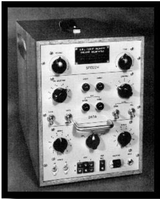
Figure 3: The playback station used for separating the cockpit speech and analysing the instrument readings.
