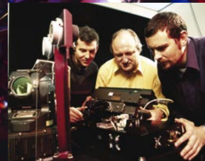
DSTO researchers William Isterling, Dr Miro Dubovinsky and Dr David Lancaster replacing commercially-developed laser in test bed with the new compact MURLIN laser.
