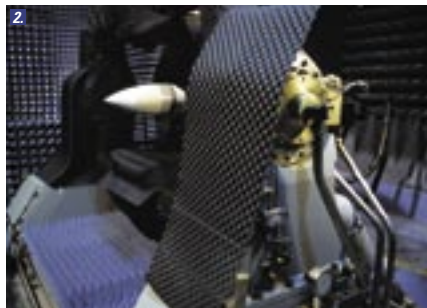
2. Simulation research setup for ESSM in DSTO's Systems Simulation Centre anechoic chamber.
